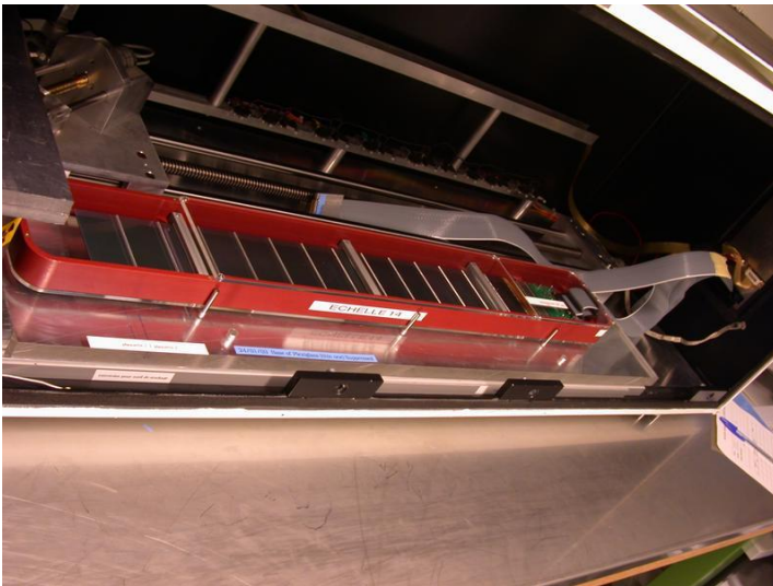
Figure 6. Example of the arrangement of the double-sided Si detectors on a ladder (part of the tracker system of AMS experiment).
