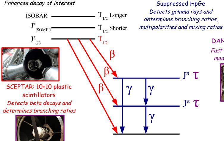
Zero-Degree Fast scintillator Fast-timing signal for betas 5
