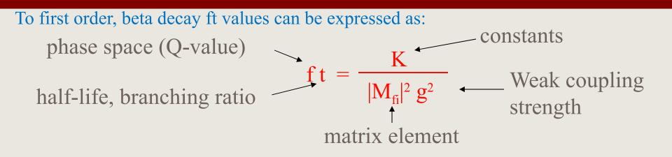
For the special case of  $0^+ \rightarrow 0^+$  (pure Fermi) beta decays between isobaric analogue states (superallowed) the matrix element is that of an isospin ladder operator:
