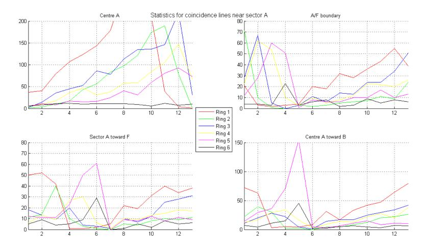
• Plots show remaining events after gating on core energy, scintillator energy, segment fold, scintillator fold and segment-scintillator matching.
