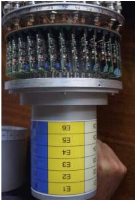
Fig. 10. 36 Preamplifier boards in situ in the detector.
