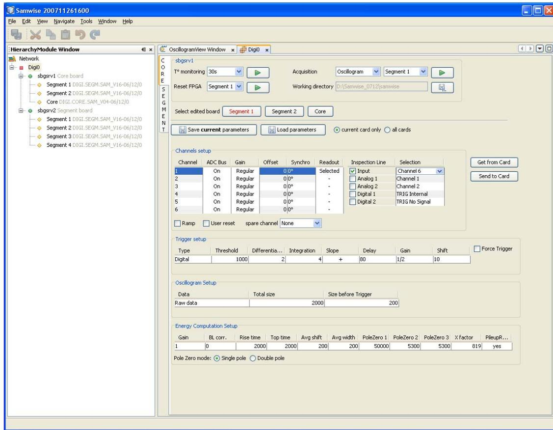
If successful you should see a sine wave. Stop acquisition, select channel 2 and enable acquisition. Repeat for all 6 channels (see snapshots below).
