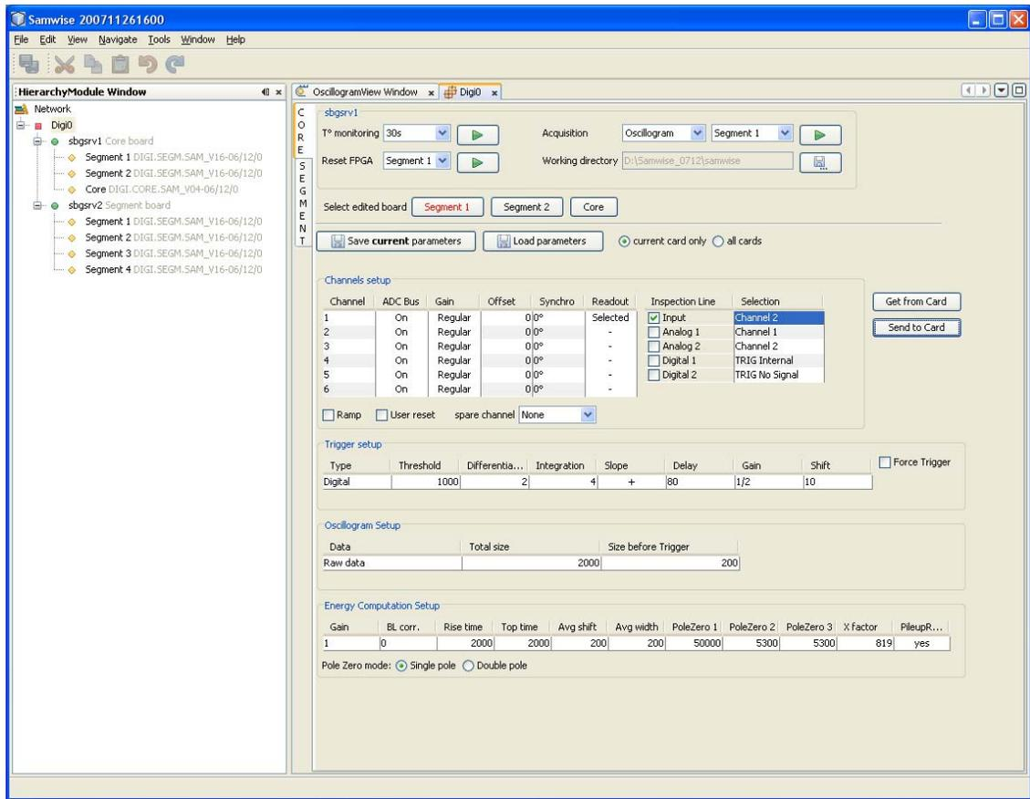
The next test is to view the sine wave of each channel in samwise. Select channel 1 as highlight below and then click on the green play icon at the top right to acquire the data for that channel:
