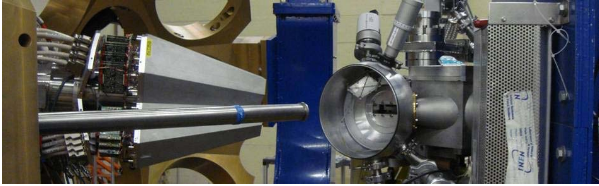
Figure 4(d)1 The experimental set-up in the Week 27 AGATA commissioning experiment. The multi-channel plate (MCP) detector of DANTE can be seen inside the target chamber.
