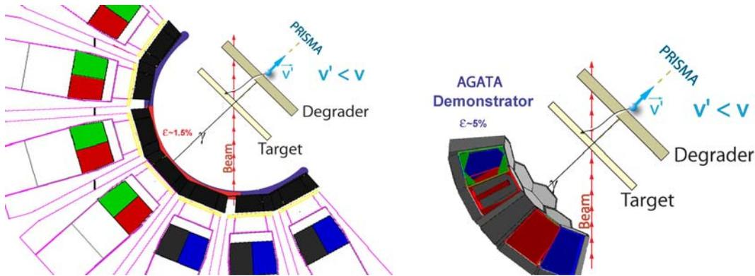
**Figure 2: Use of CLARA (left) and the Demonstrator (right) for RDDS measurements. Only half of CLARA detectors can be used for RDDS and, therefore, the effective efficiency of CLARA for RDDS is about 1.5%, compared with 5% to 6% for the Demonstrator.**
